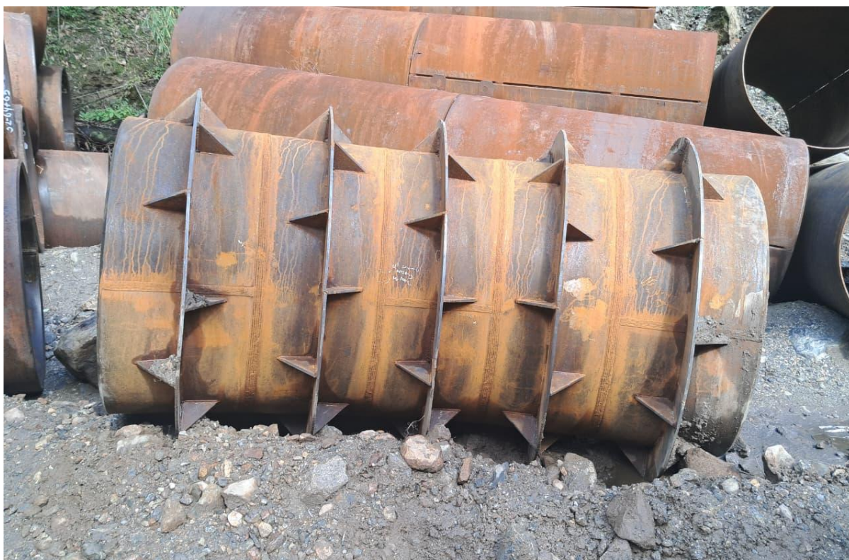
Figure 14: Anchor block 12 bend pipe
